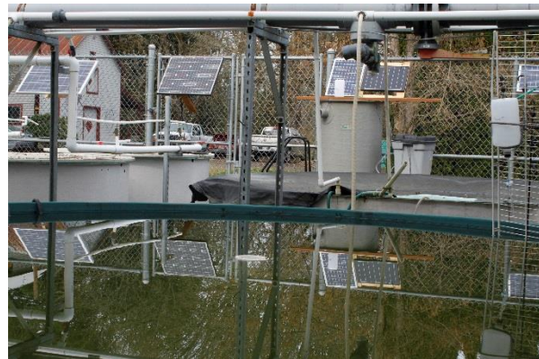
Solar panels power the students' aeration units
